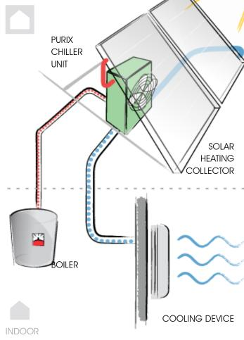
The core technology is the absorption cooling principle widely used, for instance, in refrigerators in hotel rooms due to the low noise level.
